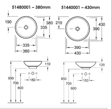
Installation Notes:  $\square$  No cut-outs should be attempted in bench top without having the actual Basin/s that are going to be installed.  $\square$  Only Silicon based adhesives should be used, not epoxy resins.  $\square$  Overflow hole should be positioned closest to the front of the cabinet.
