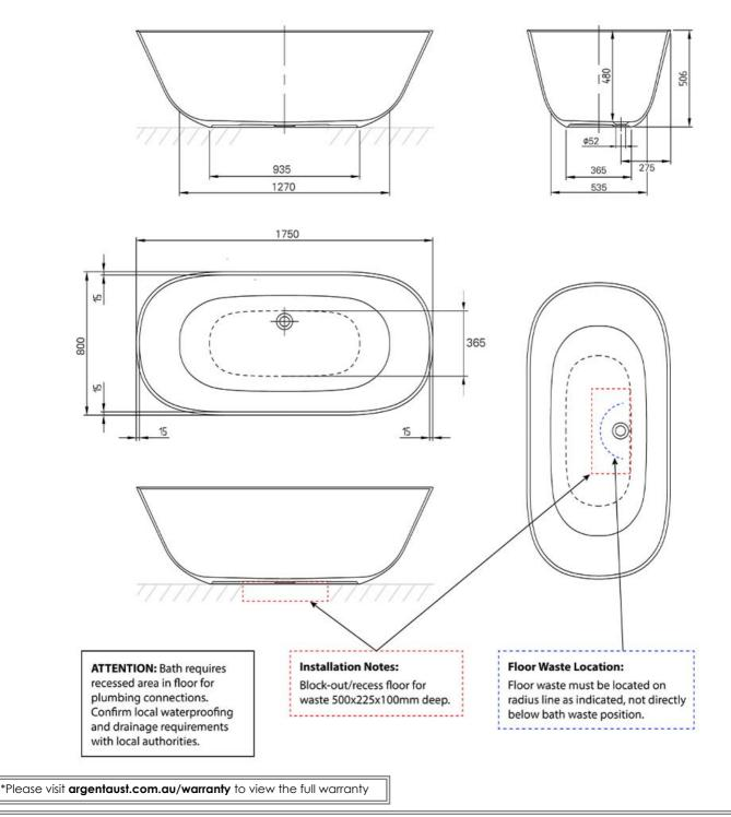
Note: All dimensions are in millimetres and are subject to normal manufacturing variations. Always use the physical product measurements for cut-outs and rough-ins as the technical details shown may differ from the actual product. Use acetic cured silicone sealant. Do not use epoxy type adhesives. Clean with damp cloth. Do not use abrasive cleaners, liquids or pastes.
