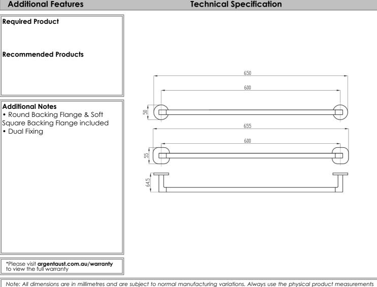
Note: All dimensions are in millimetres and are subject to normal manufacturing variations. Always use the physical product measurements for cut-outs and rough-ins as the technical details shown may differ from the actual product. Use acetic cured silicone sealant. Do not use epoxy type adhesives. Clean with damp cloth. Do not use abrasive cleaners, liquids or pastes.
