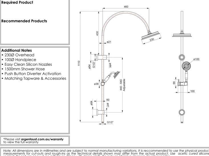
Note: All dimensions are in millimetres and are subject to normal manufacturing variations. It is reccommended to use the physical product measurements for cut-outs and rough-ins as the technical details shown may differ from the actual product. Use acetic cured silicone sealant. Do not use epoxy type adhesives. Clean with damp cloth. Do not use abrasive cleaners, liquids or pastes.
