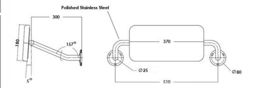
Note: All dimensions are in millimetres and are subject to normal manufacturing variations. Always use the physical product measurements for cut-outs and rough-ins as the technical details shown may differ from the actual product. Use acetic cured silicone sealant. Do not use epoxy type adhesives. Clean with damp cloth. Do not use abrasive cleaners, liquids or pastes.
