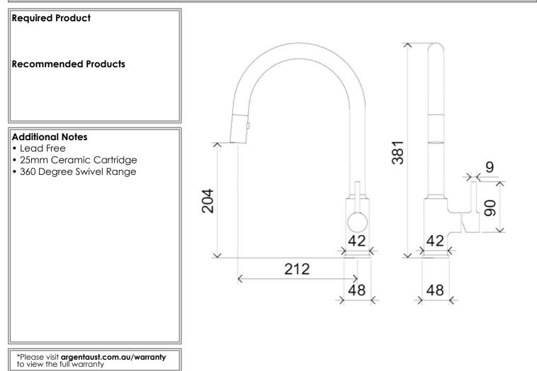
Note: All dimensions are in millimetres and are subject to normal manufacturing variations. Always use the physical product measurements for cut-outs and rough-ins as the technical details shown may differ from the actual product. Use acetic cured silicone sealant. Do not use epoxy type adhesives. Clean with damp cloth. Do not use abrasive cleaners, liquids or pastes.
